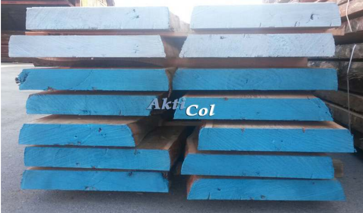
Sawn timber coated AktiCol coating for protection against cracking after one day and three hours.
